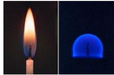
Candle flame in orbital conditions (right) versus on Earth (left)
