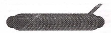
The above figure shows the image of electromagnet. Iron tack converts in to electromagnet from electricity passing through dry cell and insulating wire (aluminum foil paper) as closed circuit. Some pins were brought near the one side of iron tack. Iron tack attracted the Iron pins and needles. If the cell is disconnected no current flows in the circuit and pins fall immediately.
